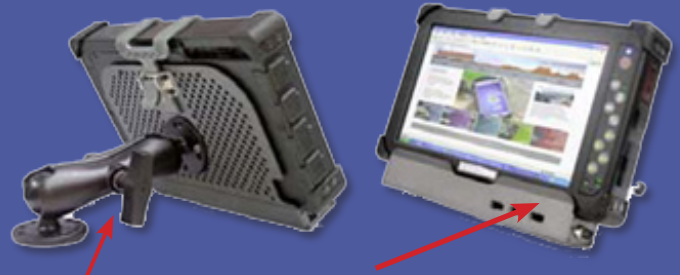
Shown with optional vehicle docking station this provides users with three additional USB ports, an RS232 serial port, a LAN port, and a DC power connection.
